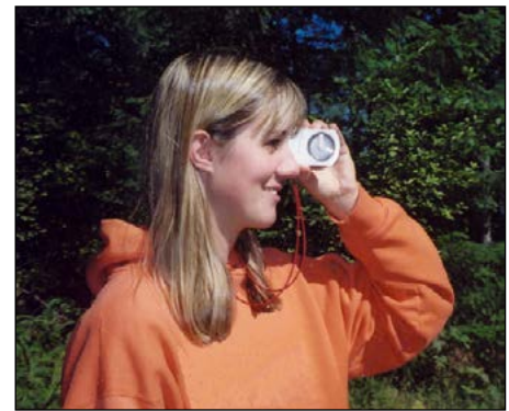
Figure 2. The clinometer has a sighting hole and a suspended circular scale that can measure ground slope as well as tree height.
