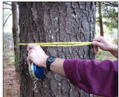
Figure 3. A combination logger's tape can measure tree diameter (above) in addition to log lengths and diameters (below).
