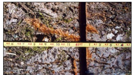
Figure 3. A combination logger's tape can measure tree diameter (above) in addition to log lengths and diameters (below).
