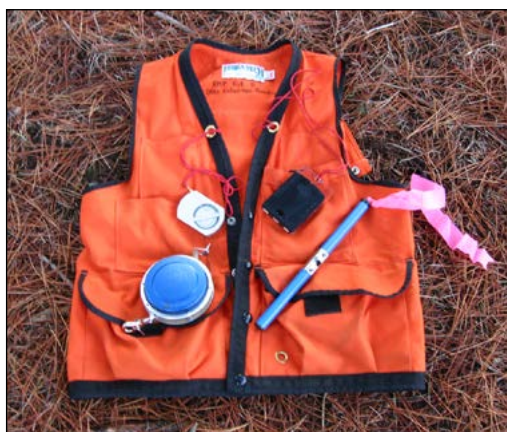
Figure 1. Tools you'll use for some measuring tasks are (clockwise, from top left) a clinometer, a compass, an increment borer (with flagging tape attached, to make the borer easier to find if it falls on the ground), and a combination logger's tape.
