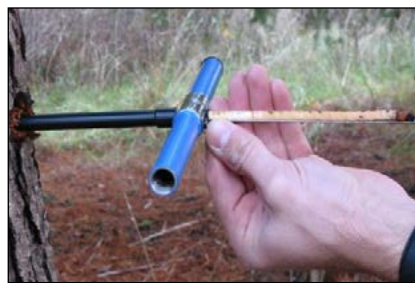
Figure 6. A core sample obtained from a tree with the increment borer allows the user to determine a tree's growth rate.
