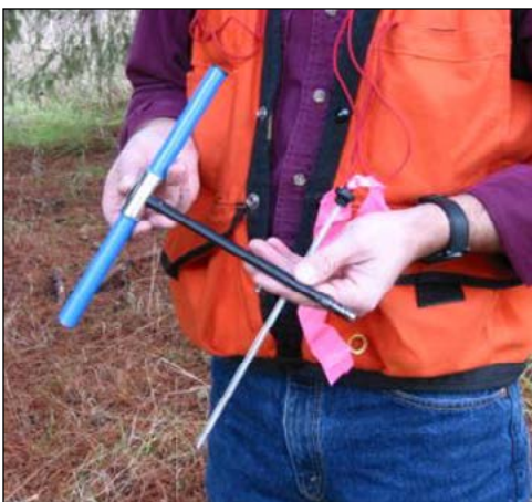
Figure 6. A core sample obtained from a tree with the increment borer allows the user to determine a tree's growth rate.
