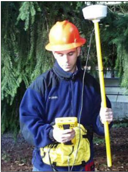
Figure 5. Consumer grade GPS units (above) are less expensive and less accurate than mapping grade GPS receivers (left), but they help make rough length or area measurements.
