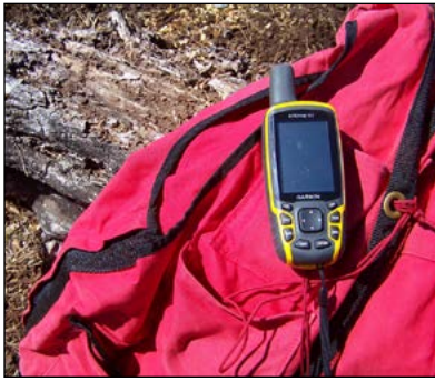
Figure 5. Consumer grade GPS units (above) are less expensive and less accurate than mapping grade GPS receivers (left), but they help make rough length or area measurements.
