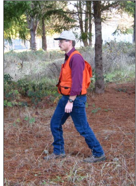
Figure 7. Pacing can be a fast, easy way to estimate area and horizontal distances. However, pacing accuracy can range widely, with results from moderately accurate to very crude. Practice in order to develop a consistent pace. You might want to buy a pedometer, such as those sold in sporting goods stores, to count your paces.
