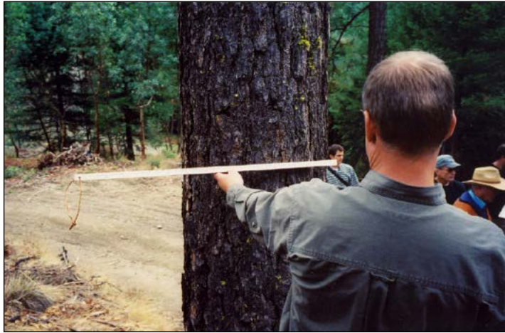
Figure 8. The Woodland Stick is an easy-to-use and moderately accurate tool for measuring tree height and diameter. It must be held 25 inches from the eye; at any other distance, it gives incorrect readings.
