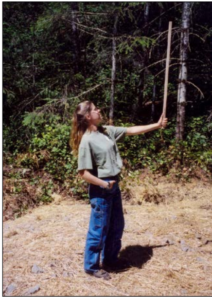
Figure 8. The Woodland Stick is an easy-to-use and moderately accurate tool for measuring tree height and diameter. It must be held 25 inches from the eye; at any other distance, it gives incorrect readings.
